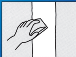
Sandpaper to a smooth finish - using a 100 grit sandpaper.
