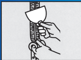
Apply RhinoTape® over RhinoBoard® joints.
