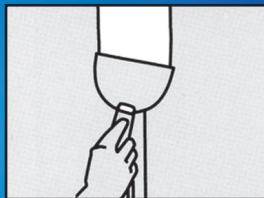
Apply RhinoGlide on top of RhinoTape® using a wide taping knife
